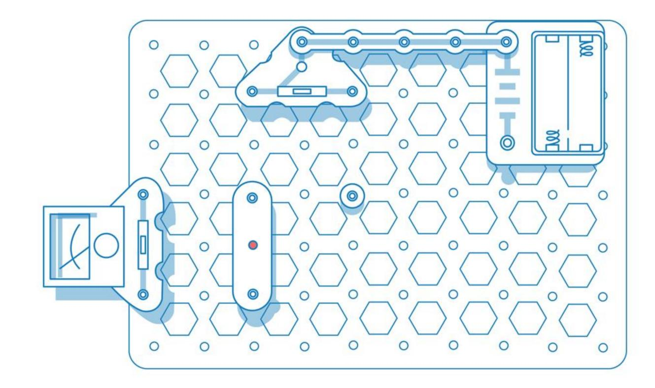
Place three of the 3-snap wires and one 1-snap wire as shown below.
