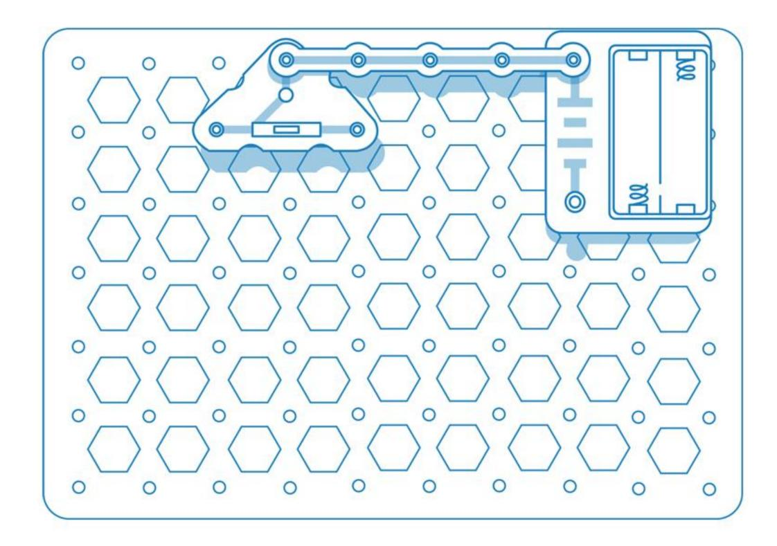
2 Snap the meter (M6), one of the LED lights, and one of the one-snap wires to the grid.
