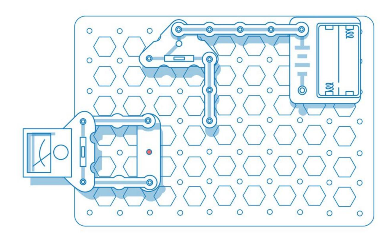
Place another 1-snap wire on top of the one already on the switch. Place a 3-snap wire and the other LED.
